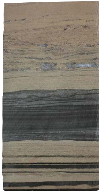
Citronen Fjord Deposit: 3.6 cm wide drill-core showing fine-grained laminated pyrite and sphalerite in black mudstone. Zinc concentration in the upper sulphide layer is 25–30% and in the lower layer 1–3%.
